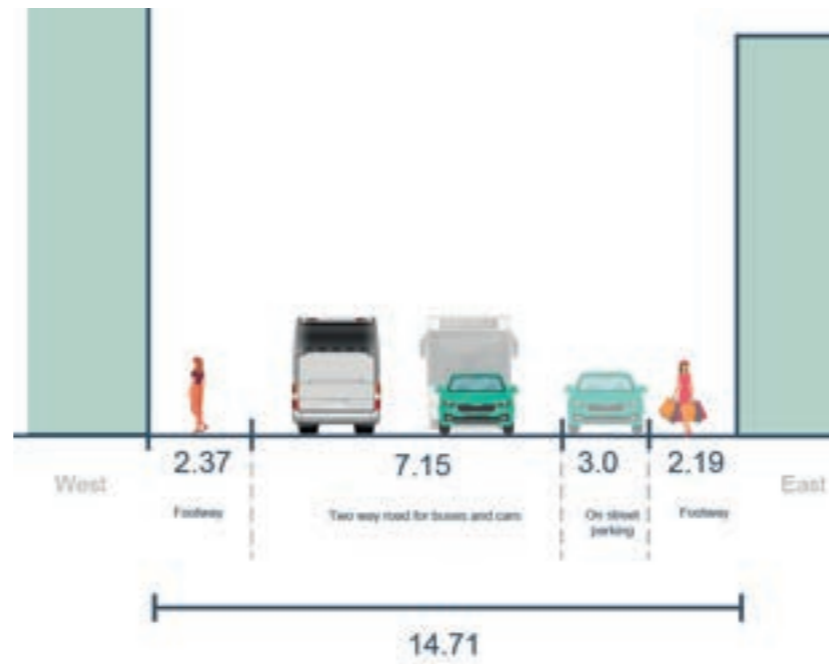
Figure 38 - Existing street section
